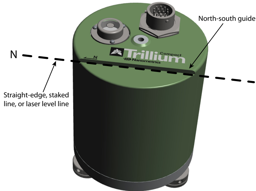
Figure 3-2 Example of seismometer alignment using the case-top guide
